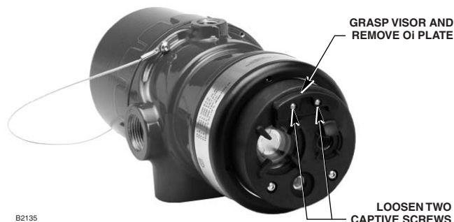
Figure 13—Oi Plate Removal
