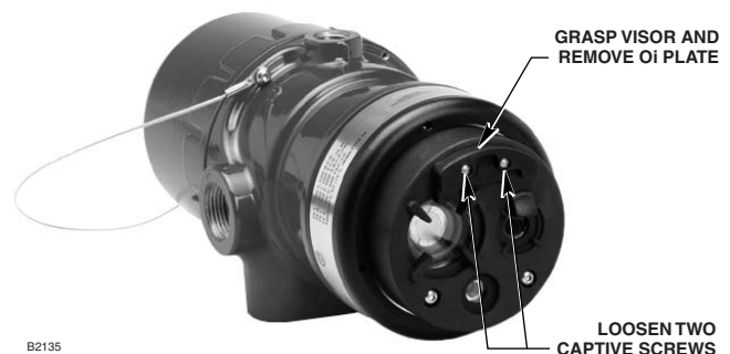
Figure 13—Oi Plate Removal
