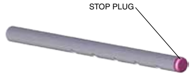
Figure 9—Inlet tube with stop plug
