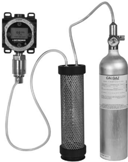
Figure 1—Calibration Setup for the NTMOS Sensor
