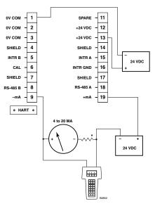
\*TOTAL LOOP RESISTANCE = 250 OHMS MINIMUM, 600 OHMS MAXIMUM. NOTE: SHIELDED CABLE RECOMMENDED (REQUIRED FOR ATEX).
