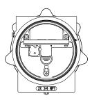
Figure 12-Terminal Strip Located Inside Wiring Compartment
