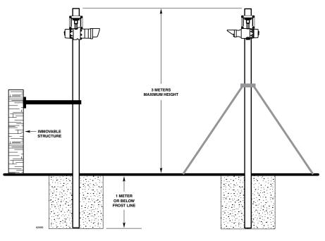
NOTE: INSTALLATIONS NEAR MAXIMUM HEIGHT TYPICALLY REQUIRE BRACING TO ENSURE NO MOVEMENT OF THE LS2000 DETECTOR.
