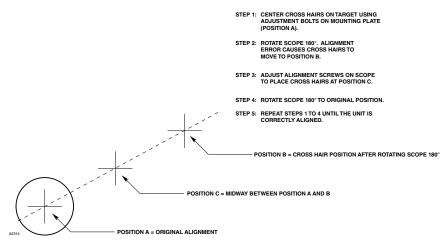
Figure 25—LS2000 Alignment Using the Telescope Alignment Tool
