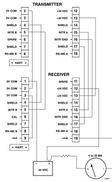
NOTE 1: TOTAL LOOP RESISTANCE OF 4-20 MA CIRCUIT = 250 OHMS MINIMUM, 600 OHMS MAXIMUM.
