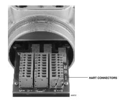
Figure 21—Location of HART Connector Pins (Receiver Module Shown)
