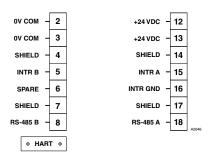
Figure 13—Transmitter Wiring Terminal Identification
