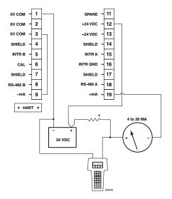
\*TOTAL LOOP RESISTANCE = 250 OHMS MINIMUM, 600 OHMS MAXIMUM. NOTE: SHIELDED CABLE RECOMMENDED (REQUIRED FOR ATEX).
