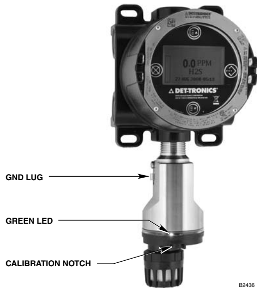
Figure 5—Correct Mounting Orientation for the GT3000
