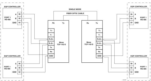
Figure 3-14—Controller to Controller NFPA 72 Approved Fiber Optic Link
