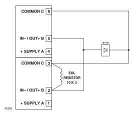
Figure 3-31—Supervised Output Configuration (Notification)— Class A, Style Z
