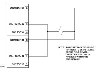
Figure 3-33—Supervised Output Configuration (Agent Release)— Class A Wiring
