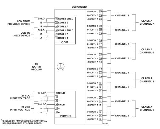
Figure 3-21—EDIO Module Wiring Terminals
