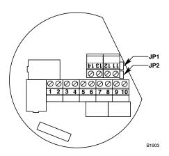
Figure 3-66—Signal Audible Module Wiring Terminals and Jumpers
