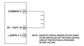
Figure 3-55—CH-7&8: Supervised Output Configuration (Agent Release)
