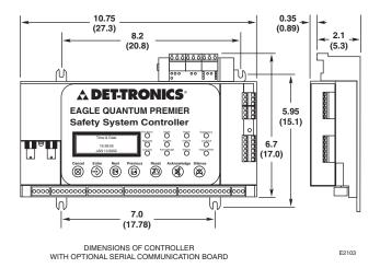
Figure 6-1—Dimensions of EQP Controller in Inches (Centimeters)
