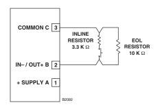
Figure 3-37—Supervised Input Configuration (Opens and Shorts)
