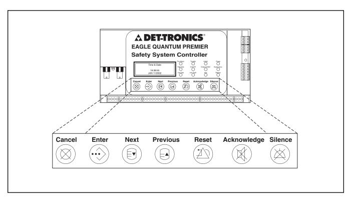
Figure 4-1—EQP Controller Pushbutton Locations
