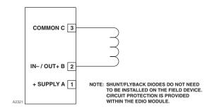
Figure 3-29—Unsupervised Output Configuration
