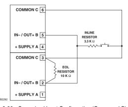
Figure 3-26—Supervised Input Configuration (Opens and Shorts) – Class A, Style E
