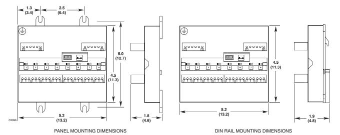
Figure 6-3—Dimensions of the EDIO / DCIO / Relay Module / AIM / IPM in Inches (Centimeters)
