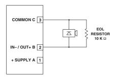
Figure 3-30—Supervised Output Configuration (Notification)— Class B, Style Y
