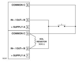
Figure 3-24—Supervised Input Configuration - Class A, Style D
