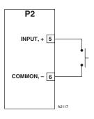
Figure 3-10—Unsupervised Input Wiring
