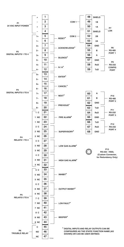
Figure 3-9—EQP Controller Terminal Identification
