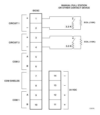
Figure 3-7—IDCSC Terminal Identification
