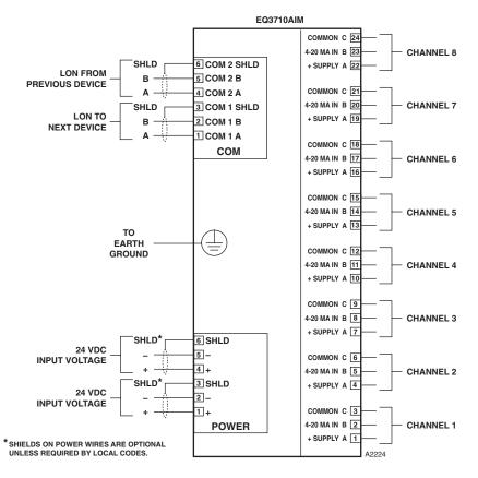
Figure 3-42—Analog Input Module Wiring Terminal Configuration
