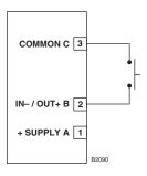
Figure 3-48—Unsupervised Input Configuration
