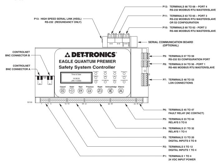
Figure 3-8—Location of Wiring Terminals on EQP Controller
