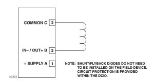
Figure 3-39—Supervised Output Configuration (Automatic Release)
