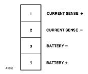
Figure 3-20—J2: Current Test Points
