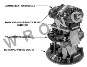
INCORRECT ORIENTATION OF TRANSMITTER BOARD
