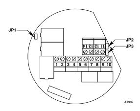
Figure 3-64—Agent Release Module Wiring Terminals and Jumpers
