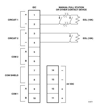
Figure 3-5—Terminal Configuration for IDC
