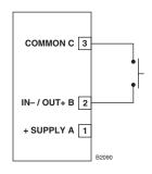
Figure 3-35—Unsupervised Input Configuration
