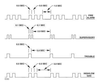
Figure 4-4—Tone Pattern for Controller Buzzer
