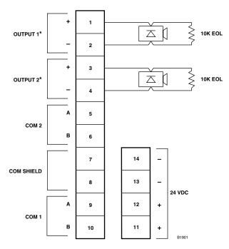
\* POLARITY SHOWN IS FOR MONITORING CONDITION, POLARITY IS REVERSED WHEN ACTIVATED.
