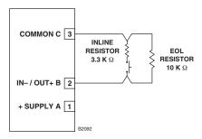
Figure 3-50—Supervised Input Configuration (Opens and Shorts)
