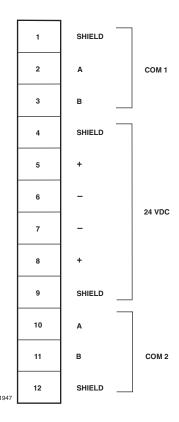
Figure 3-3—Network Extender Wiring Terminal Identification
