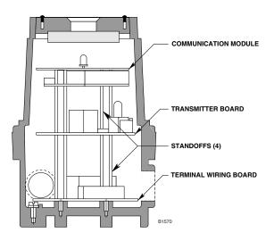
Figure 3-61—Printed Circuit Boards in Combustible Gas DCU
