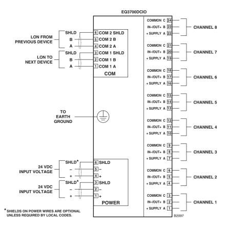
Figure 3-34—DCIO Module Wiring Terminal Configuration
