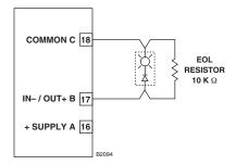
Figure 3-54—CH-6: Supervised Output Configuration (Notification)
