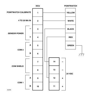
Figure 3-59—PointWatch/DuctWatch Connected to DCU
