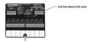
Figure 4-8—Analog Input Module Status Indicator Location
