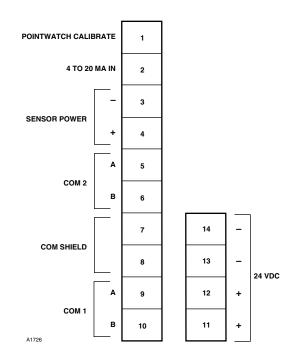
Figure 3-57—Wiring Configuration for DCU
