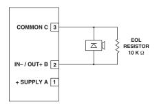
Figure 3-38—Supervised Output Configuration (Notification)
