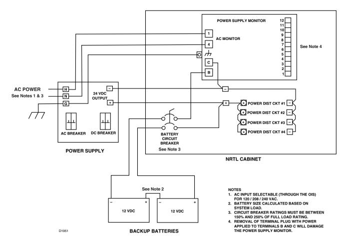
Figure 3-19— Wiring Connections for a Power Supply Monitor, Power Supply and Backup Batteries
