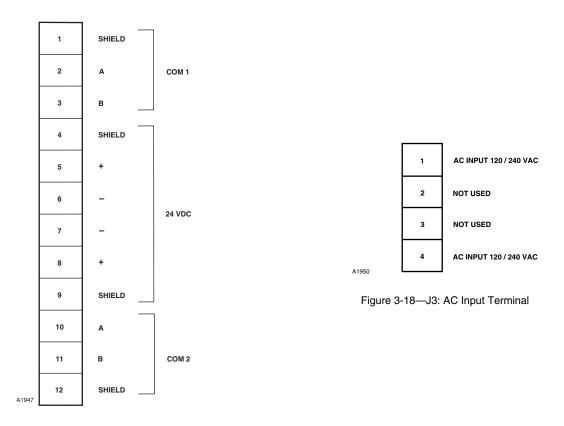
Figure 3-17—J1: Power and LON Wiring Terminal
