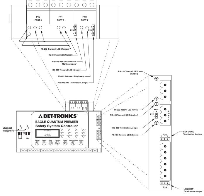
Figure 3-12—Location of Termination Jumpers, Communication Indicator LEDs and Communication Ports
