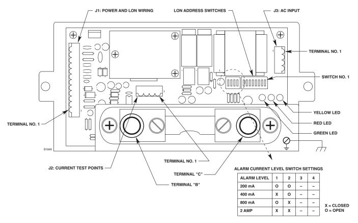
Figure 3-16—Power Supply Monitor Terminal and Switch Location
