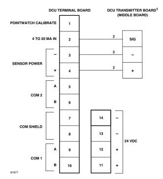
NOTES: 1 Catalytic Combustible Gas Sensor Plugs into Connector Pins on the Middle Board inside the Junction Box.
