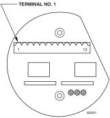
Figure 3-2—Network Extender Wiring Terminal Location
