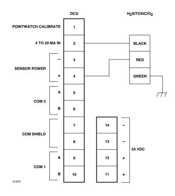
Figure 3-58—Electrochemical Sensor Connected to DCU
