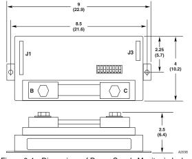
Figure 6-4—Dimensions of Power Supply Monitor in Inches (Centimeters)
