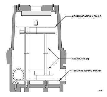
Figure 3-56—Printed Circuit Boards in Universal DCU
