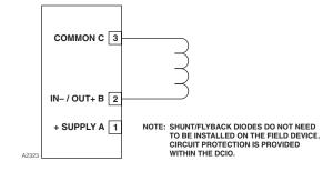
Figure 3-40—Unsupervised Output Configuration
