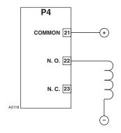
Figure 3-11—Unsupervised Relay Output
