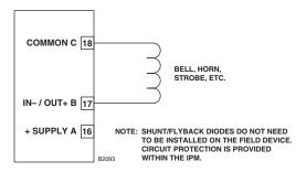
Figure 3-53—CH-6: Unsupervised Output Configuration
