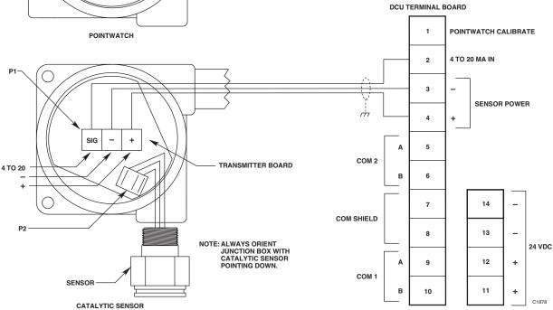
Figure 3-62—Sensor Separation Kits
