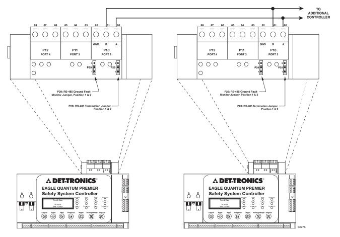
Figure 3-13—Controller to Controller Communication with Signaling Line Circuit Classification per NFPA 72
