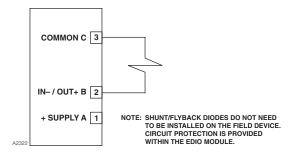
Figure 3-32—Supervised Output Configuration (Agent Release)
