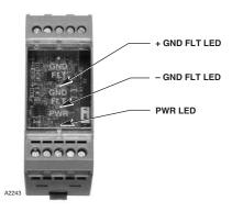
Figure 4-11—Ground Fault Monitor Status Indicator Location
