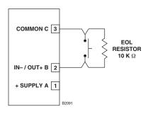
Figure 3-49—Supervised Input Configuration
