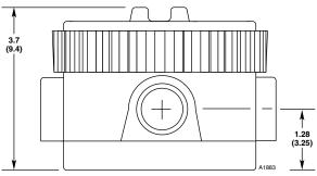
Figure 6-7—Dimensions of Short Cover Junction Box in Inches (Centimeters)
