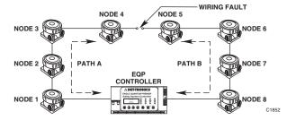
Figure 2-3—Communication over the LON with a Single Wiring Fault
