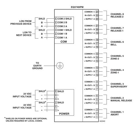
Figure 3-47—IPM Wiring Terminal Configuration
